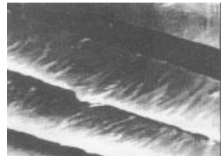
Fig. 4. SEM for the surface of Samples Treated with a mixture of PEG and Sodium hydroxide solution (95.5%/4.5% w/w) to wet pick-up of 100% expression then steaming at 160°C for 2 min; treated with CD then curing at 170°C for 2 min.
