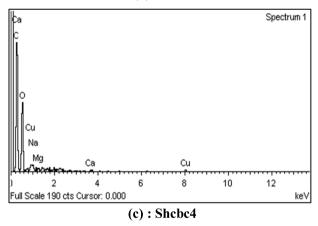
Figure 3.4: EDS graphs of untreated and treated sisal fiber
