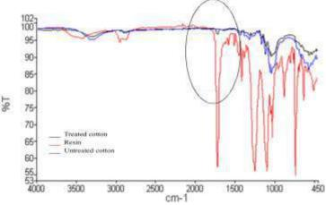
Figure 3: FTIR Spectra of treated cotton fabric, untreated cotton fabric and resin
