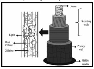
Figure 3.1: Schematic diagram of Sisal fiber cell
