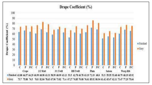
Figure 7: Drapability of grey and finished fabrics
