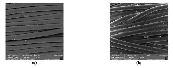
Figure 3.8 : Cordura Sample (a) before Treatment after UVA Exposure, (b) after Treatment after UVA Exposure
