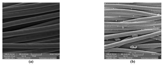
Figure 3.7 : Cordura Sample (a) before Treatment before UVA Exposure, (b) after Treatment before UVA Exposure
