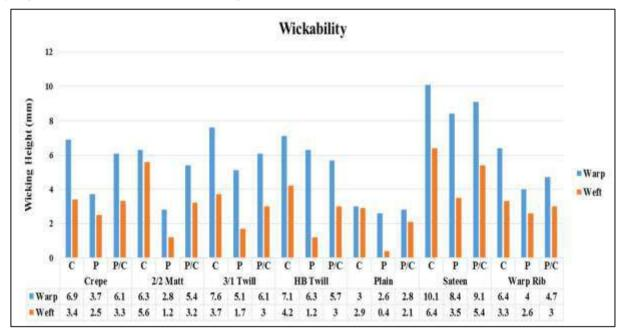
Figure 11: Wickability of grey and finished fabrics
