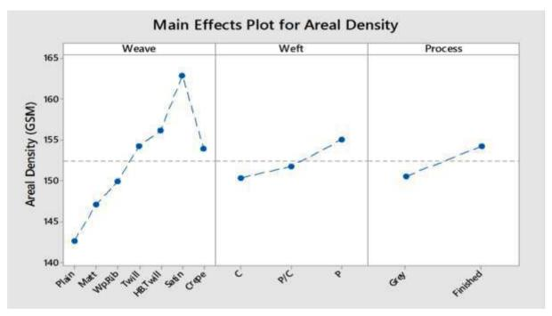
Figure 2: The effect of weave type, weft and processing on the areal density of the fabric
