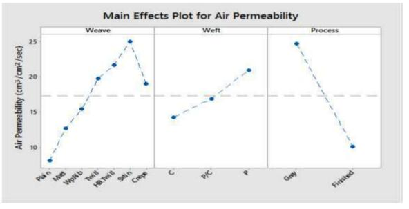
Figure 6: The effect of weave type, weft and processing on Air permeability of the fabric
