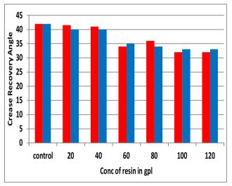
Figure 6: Crease recovery angle of treated cotton fabric
