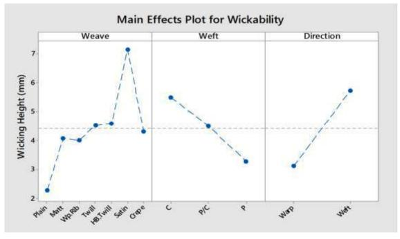
Figure 12: The effect of weave type, weft and processing on Wicking Height of fabric
