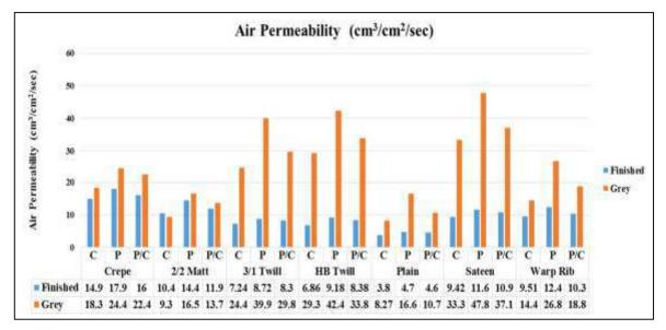
Figure 5: Air permeability of grey and finished fabrics
