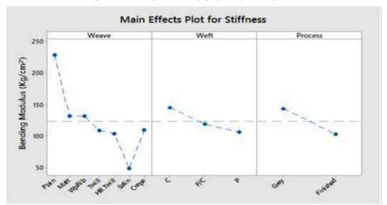
Figure 10: The effect of weave type, weft and processing on Bending modulus of fabric
