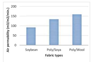
Figure 3.1 – Comparative analysis of air Permeability values of different types of fabrics
