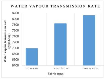
Figure 3.2: Comparative analysis of Water Vapor Transmission Rate of experimental fabrics
