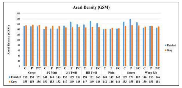
Figure 1: Areal density of grey and finished fabrics
