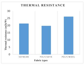
Figure 3.3 – Comparative analysis of Thermal resistance of experimental fabrics
