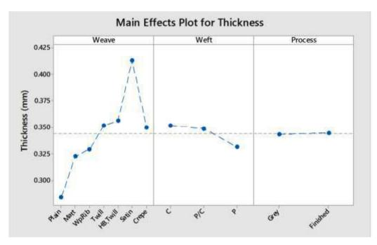
Figure 4: The effect of weave type, weft and processing on the thickness of fabric
