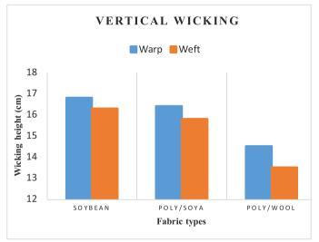
Figure 3.4 – Comparative analysis of Wickability of experimental fabrics
