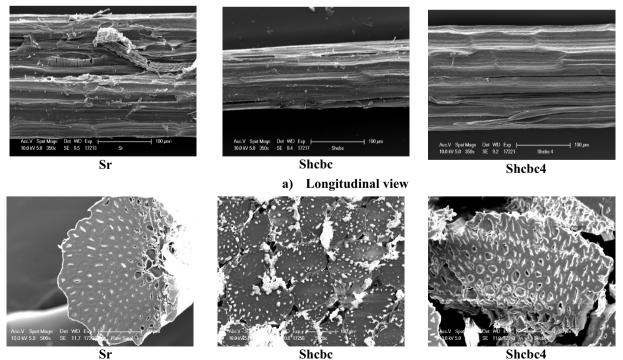
b) Cross sectional view Figure 3.2: SEM images of raw and enzyme treated fibers
