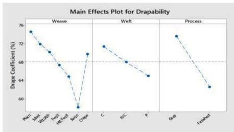
Figure 8: The effect of weave type, weft and processing on drape coefficient of fabric
