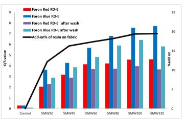
Figure 1: Add-on% and K/s Value of dyed and washed samples
