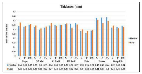
Figure 3: Thickness of grey and finished fabrics
