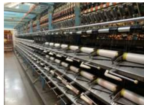
Figure 1 - Texturizing machine showing the Unit Disc and winding bobbin
