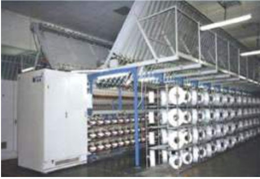
Figure 2 -Texturizing Machine with creel, heater, and 3-deck winding bobbins
