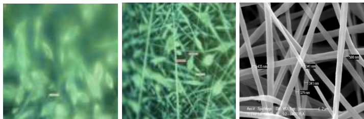
Figure 15 - PCL nanofibers by using electrospinning technique for 5, 10, 15, and 20% confocal images and scanning electrospinning microscopy images
