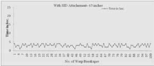
Figure 3.5: Time Vs number of warp breakages, with SID on a 63 inches loom
