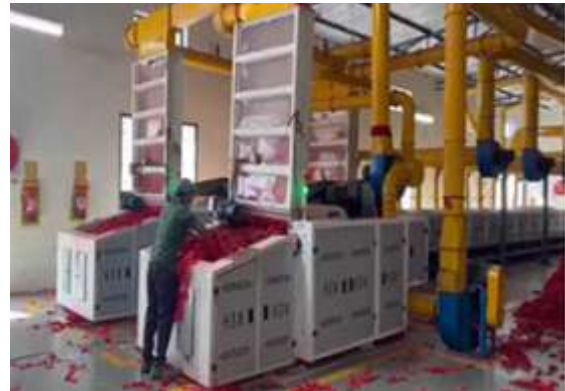
Figure 5: Shredding the color sorted clothes into fibre
