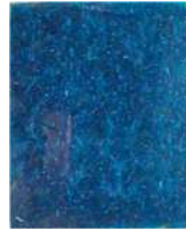
Figure 2: Composite Sheet Made Using Waste Mulberry Silk Fabric
