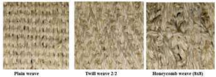
Figure 2: Plain, Twill and Honey Comb fabrics produced from Table top loom
