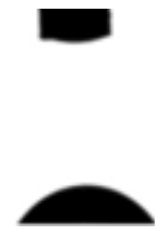
Figure 3b: Hydrophobic PU+PVC Surface contact angle=108.52°
