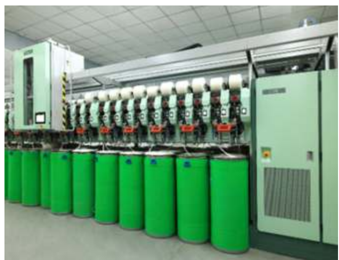
The air-jet spinning machine J 70 enables the production of high-quality yarns with maximum efficiency
