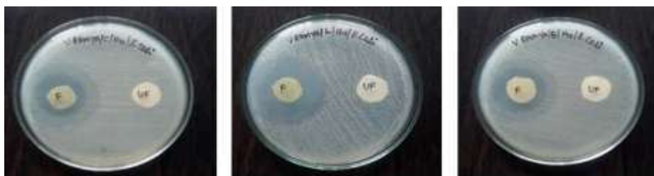
Figure 7: L. acidissima (H5) extract finished fabrics for antibacterial effectiveness against E. coli
