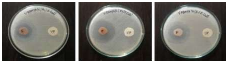
Figure 5: E. hirta (H2) extract finished fabrics for antibacterial effectiveness against E. coli
