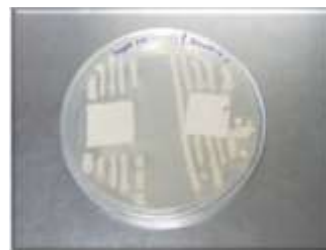
Figure 4: Activity of Neem chitosan nanoparticle against Bacillus cereus on treated cotton fabric (left) and polyester fabric (right) side of the petri dish
