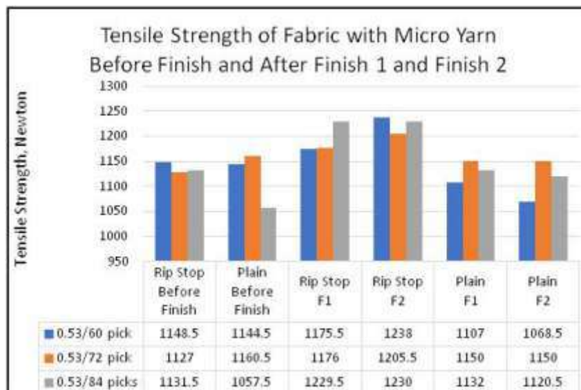
Figure 3: Tensile Strength before and after finish
