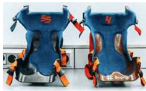
Figure 5 - McLaren F1 car seat frame – Flax prepreg
