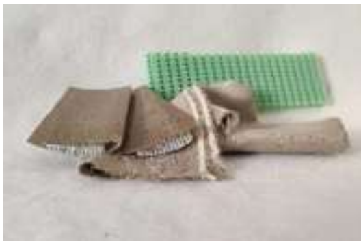
Figure 20 - Flax prepreg + PET core for Electric formula car
