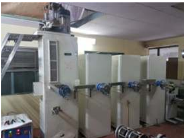
Figure 2: The pilot melt spinning machine used to develop filaments yarns
