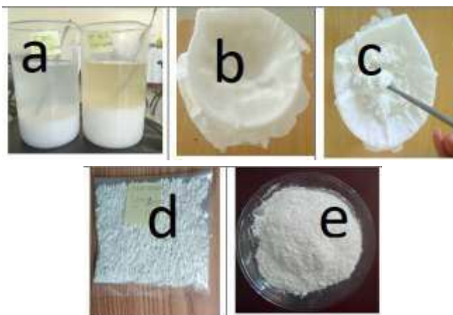
Figure 2 - The sequential extraction of waste cotton fiber (a. Treatment and hydrolysis b. Rinsing c. Filtered extract d. Dried sample, e. Fine Powder)
