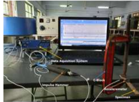
Figure - 2 Vibration testing setup
