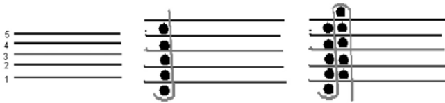
Figure 2.4: Steps for producing 3D Fabric using Orthogonal Principle
