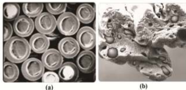
Figure 1.1: SEM of Outlast® for (a) Polyester and (b) Viscose [28].
