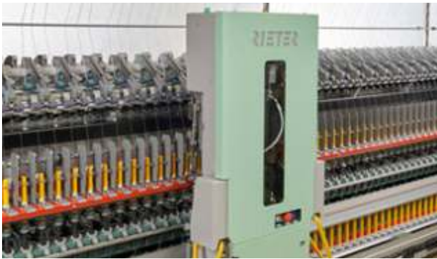
Rieter's ring spinning machine G 38 equipped with the fully automated piecing robot ROBOspin sets
