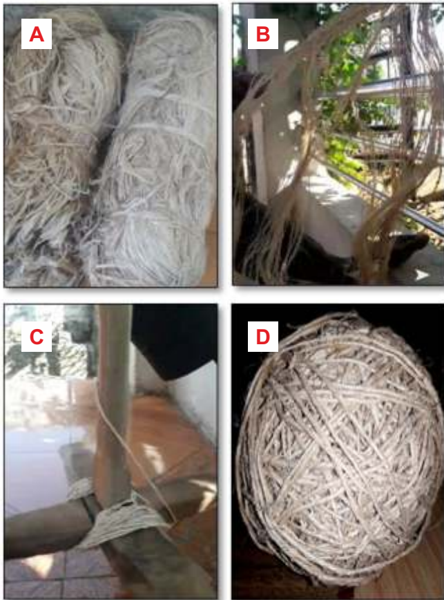
Figure 2.1 - Yarn Formation Process –A) Banana fiber bundle, B) opening and straightening of Banana fiber, C) Takli for making yarn, D) Final handmade banana yarn.
