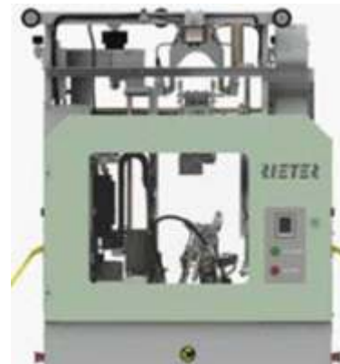
ROBOdoff automating package changes on the rotor spinning machine R 37
