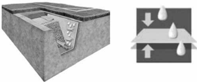
Figure 2.2 Filtration function of geotextiles
