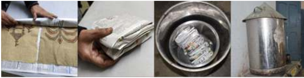
Figure 7.4: Steaming process of natural dyed and printed fabrics
